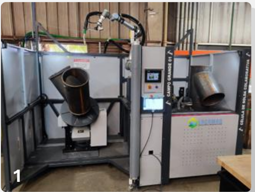
Robotic equipment for pipe welding
