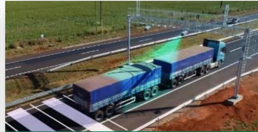
Implementation of the high-speed weigh-in-motion system (traffic enforcement from Dec/24)
