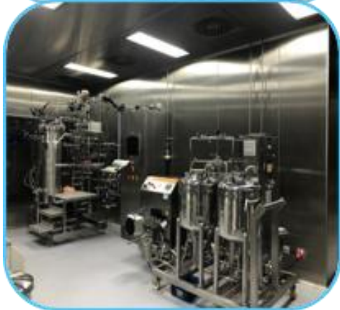
Reactors for cell culture and bacterial fermentation in the P400.
